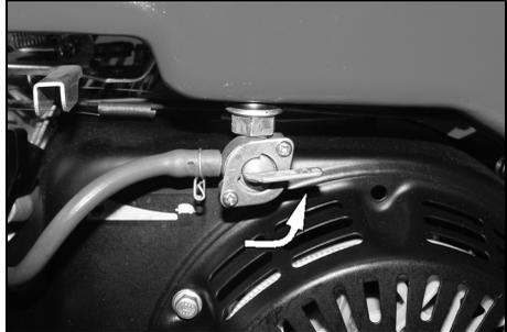
7. Rotate the trigger lock to the locked position.
