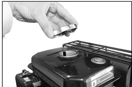
2. Pour unleaded petrol through the fuel strainer and into the fuel tank.
